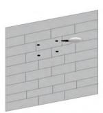
Fig. 4.2.5: Use of blow pump to loose dust from drilled holes
