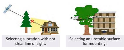
Fig. 4.1.10: Unsuitable sites for installing DTH dish
