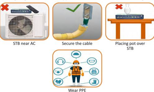
Fig. 4.3.2: Safety instructions to be followed while installing DTH
